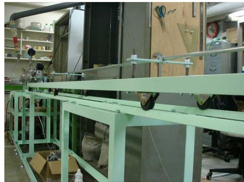
**Launch tube (Pressure vessel side)**
