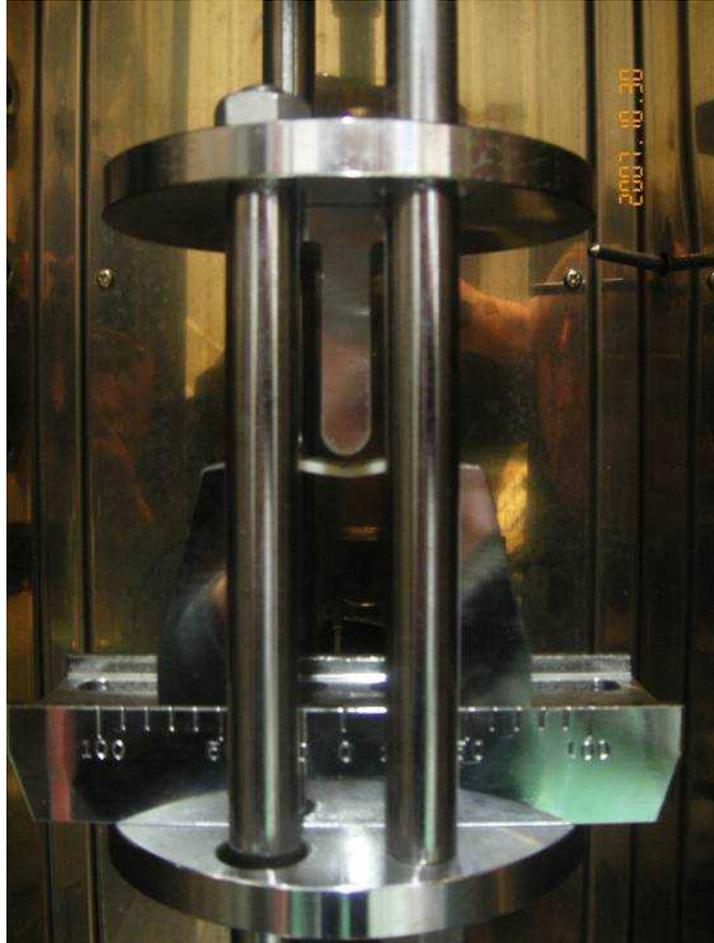
**Fig.3-2** Photograph of testing machine for flexural properties
