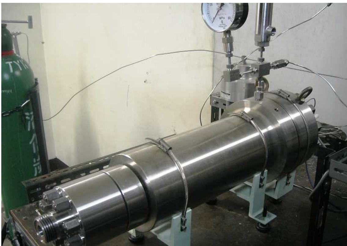
Fig.3-3 3.0ℓ pressure vessel.
