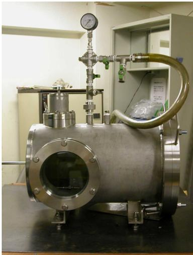
Fig.1-10 Test chamber.
