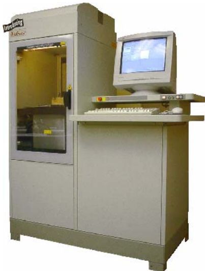
Fig.7 Viper SLA System (Microstereo Lithography)
