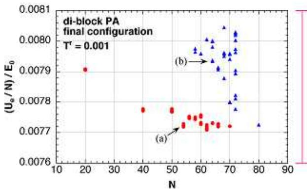
Fig. 8 Elastic potential per monomer  $U_e/N$  of the final configurations for di-block PA at  $T^r = 0.001$ .
