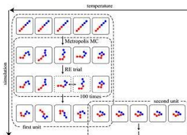
Fig. 2 Illustration of our procedure of the REMC.
