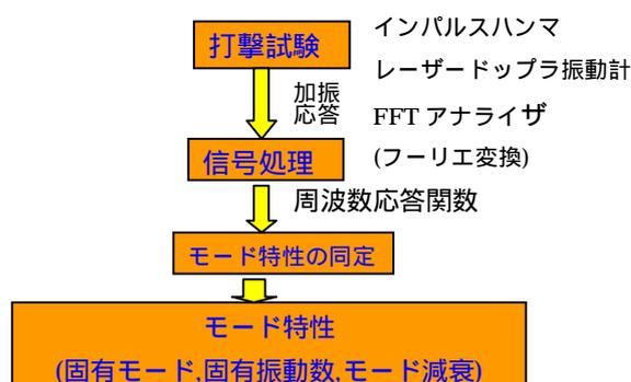
Fig.1 The method of Experimental Modal Analysis
